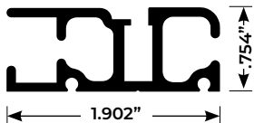
Under Track - (Small 3-Channel) XC 0092, XC 1130 (drilled)
