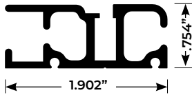
Under Track - (Small 3-Channel) XC 0092, XC 1130 (drilled)
