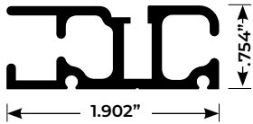
Under Track - (Small 3-Channel) XC 0092, XC 1130 (drilled)
