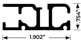
Under Track - (Small 3-Channel) XC 0092, XC 1130 (drilled)
